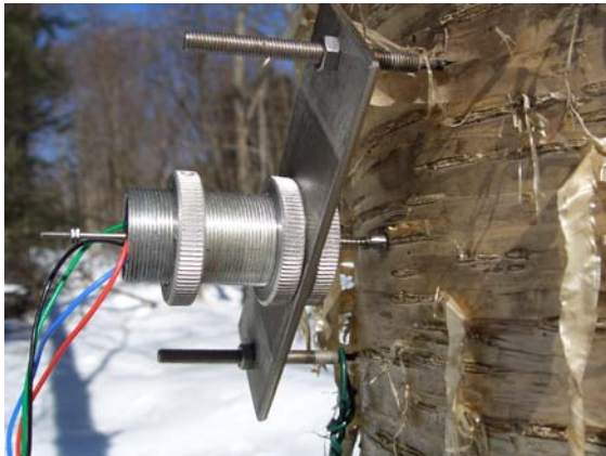
A point dendrometer on a Yellow birch in Haliburton Forest, Canada
