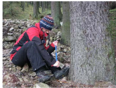
Collecting cores of Norway Spruce for dendrogeomorphological analysis of debris flows
