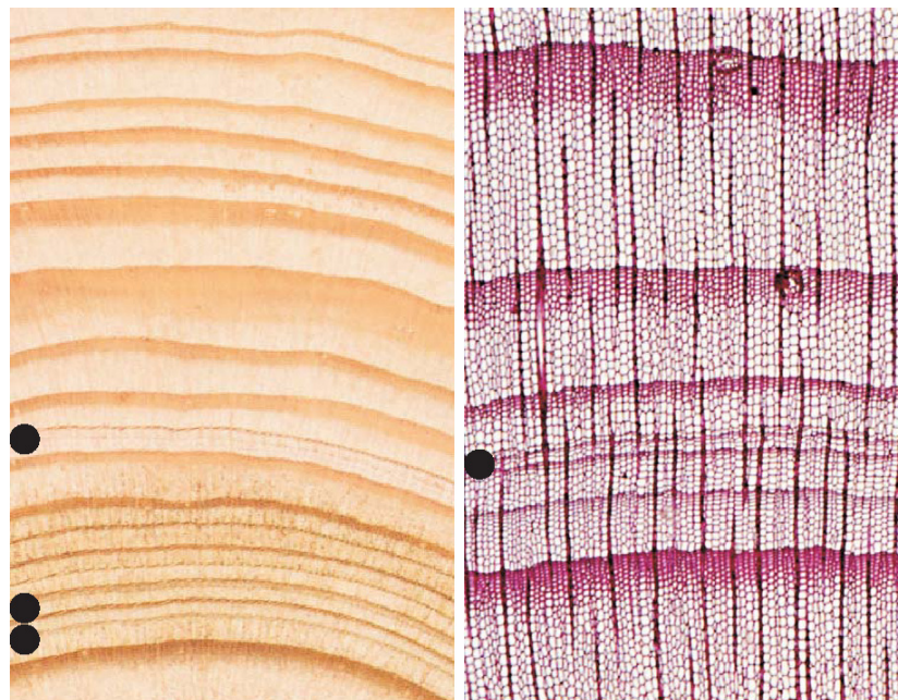
Figure 5: False rings at a site at the lower forest limit in the Turgen-Kharkhira mountains: (left) stem cross-section, (right) microsection.
