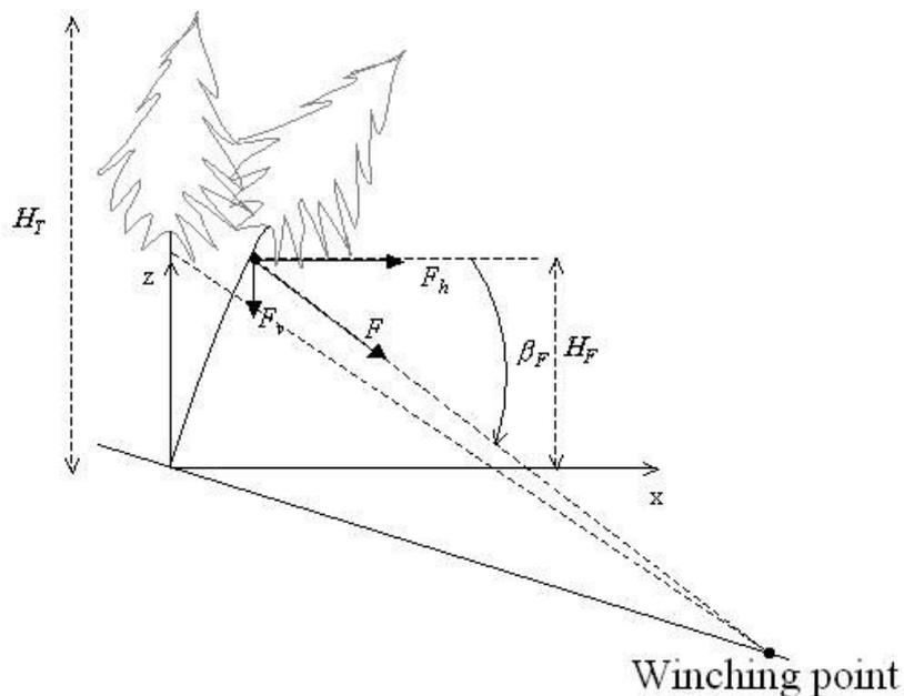
Figure 1: Test set-up of winching test.
